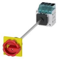
Load disconnector 3LD3, Iu 40 A Main switch 3-pole + N Rated operating capacity at AC-23 A at 400 V 18.5 kW floor mounting Basic switch with door coupling Central hole mounting 22.5mm Rotary actuator red / yellow 66 x 66 mm with auxiliary switch 1OE + 1S
