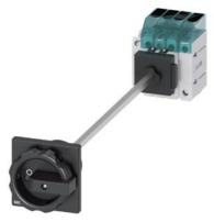
Load disconnector 3LD3, lu 40 A Main switch 3-pole + N Rated operating capacity at AC-23 A at 400 V 18.5 kW floor mounting Basic switch with door coupling Central hole mounting 22.5mm Rotating drive black 66 x 66 mm with auxiliary switch 1OE + 1S
