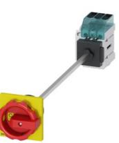
Load disconnector 3LD3, lu 40 A Main switch 3-pole Rated operating capacity at AC-23 A at 400 V 18.5 kW floor mounting Basic switch with door coupling Central hole mounting 22.5mm Rotary actuator red / yellow 66 x 66 mm with auxiliary switch 10E + 1S
