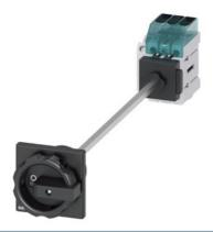
Load disconnector 3LD3, Iu 40 A Main switch 3-pole Rated operating capacity at AC-23 A at 400 V 18.5 kW floor mounting Basic switch with door coupling Central hole mounting 22.5mm Rotating drive black 66 x 66 mm with auxiliary switch 1OE  $\pm$  1S
