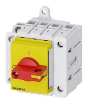
Load disconnector 3LD3, Iu 40 A Main switch 3-pole + N Rated operating capacity at AC-23 A at 400 V 18.5 kW Installation in distribution boards, Basic switch with selector knob red / yellow with auxiliary switch 10E + 1S
