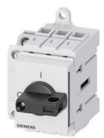
Load disconnector 3LD3, lu 40 A Main switch 3-pole Rated operating capacity at AC-23 A at 400 V 18.5 kW Installation in distribution boards, Basic switch with selector knob black with auxiliary switch 10E + 1S
