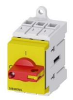
Load disconnector 3LD3, lu 40 A Main switch 3-pole Rated operating capacity at AC-23 A at 400 V 18.5 kW Installation in distribution boards, Basic switch with selector knob red / yellow
