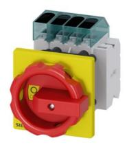
Load disconnector 3LD3, lu 32 A Main switch 3-pole + N Rated operating capacity for AC-23 A at 400V 11.5kW Front plate mounting Basic switch with Central hole mounting 22.5mm Rotary actuator red / yellow 66 x 66 mm with auxiliary switch 1OE + 1S
