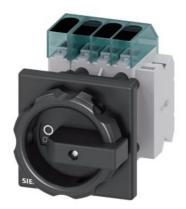
Load disconnector 3LD3, Iu 32 A Main switch 3-pole + N Rated operating capacity for AC-23 A at 400V 11.5kW Front plate mounting Basic switch with Central hole mounting 22.5mm Rotating drive black 66 x 66 mm with auxiliary switch 1OE + 1S
