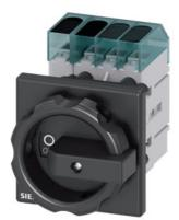
Load disconnector 3LD3, lu 32 A Main switch 3-pole + N Rated operating capacity for AC-23 A at 400V 11.5kW Front plate mounting Basic switch with Central hole mounting 22.5mm Rotating drive black 66 x 66 mm
