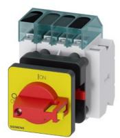
Load disconnector 3LD3, lu 32 A Main switch 3-pole + N Rated operating capacity for AC-23 A at 400V 11.5kW Front plate mounting Basic switch with Central hole mounting 22.5mm Toggle drive red / yellow 48x48 mm with auxiliary switch 10E + 1S
