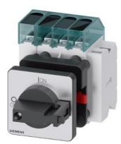
Load disconnector 3LD3, lu 32 A Main switch 3-pole + N Rated operating capacity for AC-23 A at 400V 11.5kW Front plate mounting Basic switch with Central hole mounting 22.5mm Toggle drive black 48x48 mm with auxiliary switch 1OE + 1S
