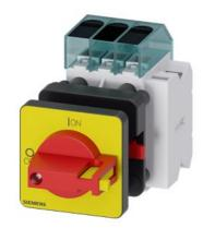
Load disconnector 3LD3, lu 32 A Main switch 3-pole Rated operating capacity for AC-23 A at 400V 11.5kW Front plate mounting Basic switch with Central hole mounting 22.5mm Toggle drive red / yellow 48x48 mm with auxiliary switch 1OE + 1S
