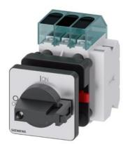
Load disconnector 3LD3, lu 32 A Main switch 3-pole Rated operating capacity for AC-23 A at 400V 11.5kW Front plate mounting Basic switch with Central hole mounting 22.5mm Toggle drive black 48x48 mm with auxiliary switch 1OE + 1S
