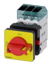
Load disconnector 3LD3, Iu 32 A Main switch 3-pole Rated operating capacity for AC-23 A at 400V 11.5kW Front plate mounting Basic switch with Central hole mounting 22.5mm Toggle drive red / yellow 48x48 mm
