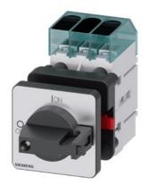
Load disconnector 3LD3, lu 32 A Main switch 3-pole Rated operating capacity for AC-23 A at 400V 11.5kW Front plate mounting Basic switch with Central hole mounting 22.5mm Toggle drive black 48x48 mm
