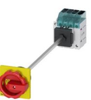
Load disconnector 3LD3, lu 32 A Main switch 3-pole + N Rated operating capacity for AC-23 A at 400V 11.5kW floor mounting Basic switch with door coupling Central hole mounting 22.5mm Rotary actuator red / yellow 66 x 66 mm with auxiliary switch 10E + 1S
