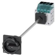
Load disconnector 3LD3, Iu 32 A Main switch 3-pole + N Rated operating capacity for AC-23 A at 400V 11.5kW floor mounting Basic switch with door coupling Central hole mounting 22.5mm Rotating drive black 66 x 66 mm with auxiliary switch 10E + 1S
