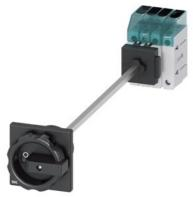
Load disconnector 3LD3, Iu 32 A Main switch 3-pole + N Rated operating capacity for AC-23 A at 400V 11.5kW floor mounting Basic switch with door coupling Central hole mounting 22.5mm Rotating drive black 66 x 66 mm
