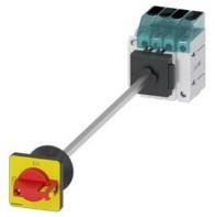
Load disconnector 3LD3, Iu 32 A Main switch 3-pole + N Rated operating capacity for AC-23 A at 400V 11.5kW floor mounting Basic switch with door coupling Central hole mounting 22.5mm Toggle drive red / yellow 48x48 mm with auxiliary switch 1OE + 1S
