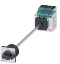
Load disconnector 3LD3, lu 32 A Main switch 3-pole + N Rated operating capacity for AC-23 A at 400V 11.5kW floor mounting Basic switch with door coupling Central hole mounting 22.5mm Toggle drive black 48x48 mm with auxiliary switch 1OE + 1S
