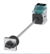
Load disconnector 3LD3, lu 32 A Main switch 3-pole Rated operating capacity for AC-23 A at 400V 11.5kW floor mounting Basic switch with door coupling Central hole mounting 22.5mm Toggle drive black 48x48 mm with auxiliary switch 10E + 1S
