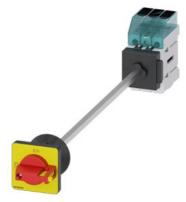
Load disconnector 3LD3, Iu 32 A Main switch 3-pole Rated operating capacity for AC-23 A at 400V 11.5kW floor mounting Basic switch with door coupling Central hole mounting 22.5mm Toggle drive red / yellow 48x48 mm
