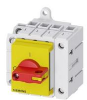
Load disconnector 3LD3, Iu 32 A Main switch 3-pole + N Rated operating capacity for AC-23 A at 400V 11.5kW Installation in distribution boards, Basic switch with selector knob red / yellow with auxiliary switch 1OE + 1S
