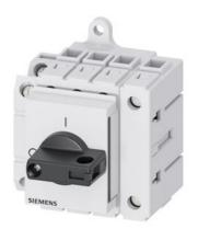
Load disconnector 3LD3, Iu 32 A Main switch 3-pole + N Rated operating capacity for AC-23 A at 400V 11.5kW Installation in distribution boards, Basic switch with selector knob black with auxiliary switch 10E + 1S
