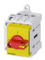
Load disconnector 3LD3, Iu 32 A Main switch 3-pole Rated operating capacity for AC-23 A at 400V 11.5kW Installation in distribution boards, Basic switch with selector knob red / yellow with auxiliary switch 1OE + 1S
