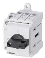
Load disconnector 3LD3, Iu 32 A Main switch 3-pole Rated operating capacity for AC-23 A at 400V 11.5kW Installation in distribution boards, Basic switch with selector knob black with auxiliary switch 10E + 1S
