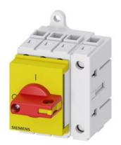
Load disconnector 3LD3, Iu 32 A Main switch 3-pole + N Rated operating capacity for AC-23 A at 400V 11.5kW Installation in distribution boards, Basic switch with selector knob red / yellow
