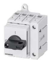
Load disconnector 3LD3, lu 32 A Main switch 3-pole + N Rated operating capacity for AC-23 A at 400V 11.5kW Installation in distribution boards, Basic switch with selector knob black
