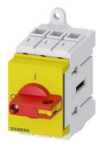
Load disconnector 3LD3, Iu 32 A Main switch 3-pole Rated operating capacity for AC-23 A at 400V 11.5kW Installation in distribution boards, Basic switch with selector knob red / yellow
