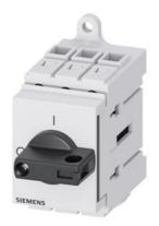
Load disconnector 3LD3, lu 32 A Main switch 3-pole Rated operating capacity for AC-23 A at 400V 11.5kW Installation in distribution boards, Basic switch with selector knob black
