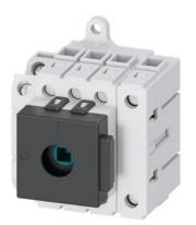
Load disconnector 3LD3, Iu 32 A Main switch 3-pole + N Rated operating capacity for AC-23 A at 400V 11.5kW Installation in distribution boards, Basic switch without Knob-operated mechanism with auxiliary switch 1OE + 1S
