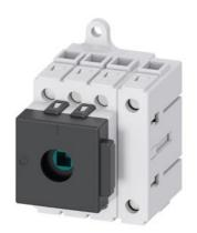
Load disconnector 3LD3, Iu 32 A Main switch 3-pole + N Rated operating capacity for AC-23 A at 400V 11.5kW Installation in distribution boards, Basic switch without Knob-operated mechanism
