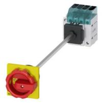
Load disconnector 3LD3, Iu 25 A Main switch 3-pole + N Rated operating capacity at AC-23 A at 400V 9.0kW floor mounting Basic switch with door coupling Central hole mounting 22.5mm Rotary actuator red / yellow 66 x 66 mm with auxiliary switch 10E + 1S
