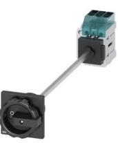
Load disconnector 3LD3, lu 25 A Main switch 3-pole Rated operating capacity at AC-23 A at 400V 9.0kW floor mounting Basic switch with door coupling Central hole mounting 22.5mm Rotating drive black 66 x 66 mm with auxiliary switch 1OE + 1S
