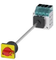
Load disconnector 3LD3, lu 25 A Main switch 3-pole + N Rated operating capacity at AC-23 A at 400V 9.0kW floor mounting Basic switch with door coupling Central hole mounting 22.5mm Toggle drive red / yellow 48x48 mm with auxiliary switch 10E + 1S
