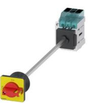
Load disconnector 3LD3, lu 25 A Main switch 3-pole Rated operating capacity at AC-23 A at 400V 9.0kW floor mounting Basic switch with door coupling Central hole mounting 22.5mm Toggle drive red / yellow 48x48 mm with auxiliary switch 10E + 1S
