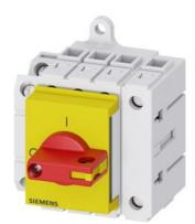
Load disconnector 3LD3, Iu 25 A Main switch 3-pole + N Rated operating capacity at AC-23 A at 400V 9.0kW Installation in distribution boards, Basic switch with selector knob red / yellow with auxiliary switch 10E + 1S
