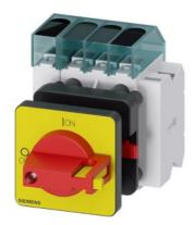
Load disconnector 3LD3, lu 16 A Main switch 3-pole + N Rated operating capacity at AC-23 A at 400V 7.5kW Front plate mounting Basic switch with Central hole mounting 22.5mm Toggle drive red / yellow 48x48 mm with auxiliary switch 10E + 1S
