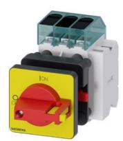
Load disconnector 3LD3, Iu 16 A Main switch 3-pole Rated operating capacity at AC-23 A at 400V 7.5kW Front plate mounting Basic switch with Central hole mounting 22.5mm Toggle drive red / yellow 48x48 mm with auxiliary switch 1OE + 1S
