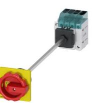
Load disconnector 3LD3, lu 16 A Main switch 3-pole + N Rated operating capacity at AC-23 A at 400V 7.5kW floor mounting Basic switch with door coupling Central hole mounting 22.5mm Rotary actuator red / yellow 66 x 66 mm with auxiliary switch 1OE + 1S
