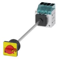
Load disconnector 3LD3, Iu 16 A Main switch 3-pole + N Rated operating capacity at AC-23 A at 400V 7.5kW floor mounting Basic switch with door coupling Central hole mounting 22.5mm Toggle drive red / yellow 48x48 mm with auxiliary switch 10E+1S
