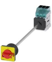
Load disconnector 3LD3, lu 16 A Main switch 3-pole Rated operating capacity at AC-23 A at 400V 7.5kW floor mounting Basic switch with door coupling Central hole mounting 22.5mm Toggle drive red / yellow 48x48 mm
