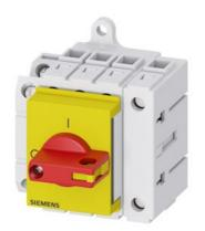
Load disconnector 3LD3, Iu 16 A Main switch 3-pole + N Rated operating capacity at AC-23 A at 400V 7.5kW Installation in distribution boards, Basic switch with selector knob red / yellow with auxiliary switch 10E + 1S
