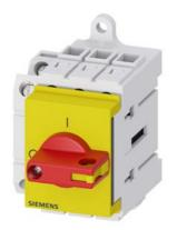
Load disconnector 3LD3, Iu 16 A Main switch 3-pole Rated operating capacity at AC-23 A at 400V 7.5kW Installation in distribution boards, Basic switch with selector knob red / yellow with auxiliary switch 1OE + 1S
