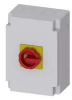
SENTRON, Switch disconnector 3LD, emergency switching-off switch, 3- pole, lu: 125 A, operating power / at AC-23 A 400 V: 45 kW, Molded plastic encapsulation for inch cable gland, 1 NC, 1 NO, rotary operating mechanism, red/yellow
