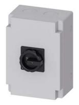
SENTRON, Switch disconnector 3LD, main switch, 3-pole, lu: 125 A, Operating power / at AC-23 A at 400 V: 45 kW, molded-plastic encapsulation for inch cable gland, 1 NC, 1 NO, rotary operating mechanism, black
