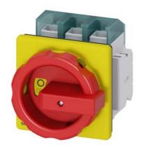
SENTRON, Switch disconnector 3LD, emergency switching-off switch, 3- pole, lu: 125 A, operating power / at AC-23 A 400 V: 45 kW, front-mounted, 1 NC, 1 NO, rotary operating mechanism, Red / yellow, 4-hole mounting of the handle
