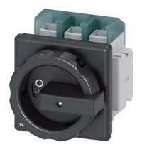
SENTRON, Switch disconnector 3LD, main switch, 3-pole, lu: 125 A, Operating power / at AC-23 A at 400 V: 45 kW, front-mounted, 1 NC, 1 NO, rotary operating mechanism, black, 4-hole mounting of the handle
