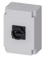
SENTRON, Switch disconnector 3LD, main switch, 3-pole, lu: 100 A, Operating power / at AC-23 A at 400 V: 37 kW, molded-plastic encapsulation for inch cable gland, 1 NC, 1 NO, rotary operating mechanism, black
